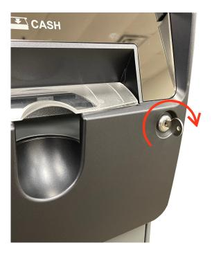
For Through the Wall ATM models, there will be a cabinet lock on the rear side of the ATM to access the internal components and Rear Service Panel.
