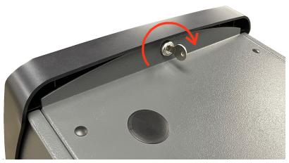
There is a second lock on the lower section of the ATM which covers the safe door lock. Use the same key to open the lower or vault bezel lock.
